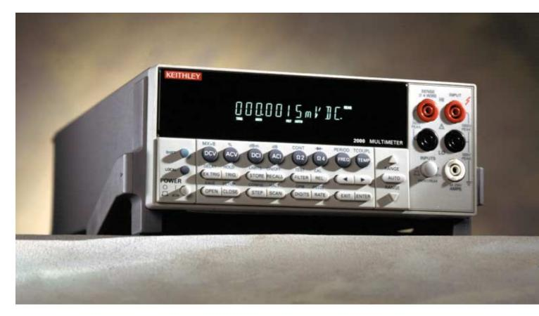
Using a precision, low-cost A-to-D converter enabled the Model 2000 design team to develop a unique error reduction algorithm. This algorithm corrects for drift errors associated with the resistor networks used for signal conditioning. Therefore, it allows the use of inexpensive resistor networks, while providing higher accuracy.
