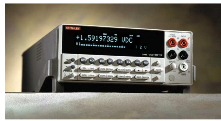
The Model 2002 offers a variety of advantages over other 8½-digit measurement instruments of comparable accuracy, particularly its DC volts and resistance measurement capabilities. For example, its measurement performance is specified for  $a \pm 5^{\circ}C$  environment, not  $a \pm 1^{\circ}C$  environment like many others, and its performance is specified for a wide range of measurement speeds. Also, it does not require a daily re-calibration to
